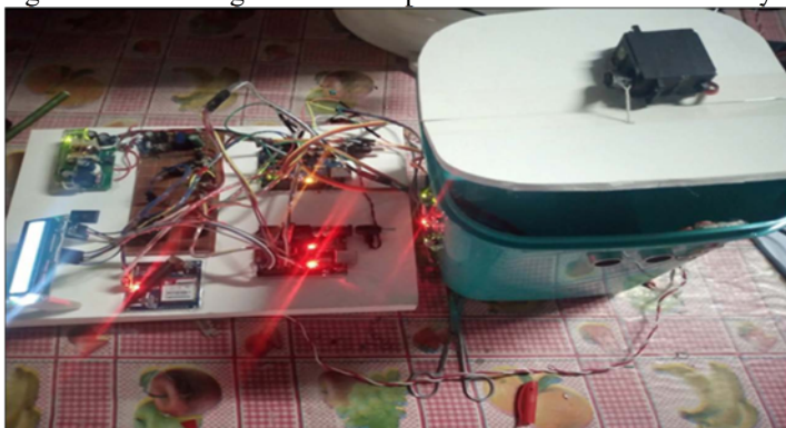
Figure 5: Circuits inside an implemented Smart sBin
