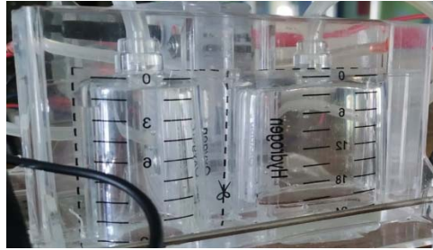
Figure 3.2. Hydrogen and oxygen gas are separately stored in two tanks
