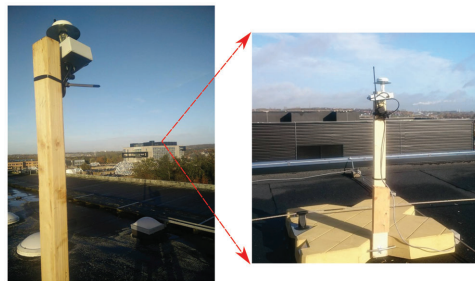
Figure 6 ublox M8P base ( left ) and rover ( right ) mounted on rooftop of Aalborg University buildings. The spatial separation between the rooftop of base and rover is 160 m.
