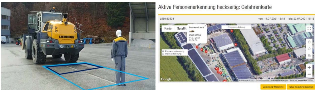
Figure 3: Left: Wheel loader with smart pedestrian detection (approximate warning zones for obstacles and pedestrians highlighted). Right: Online incident map
