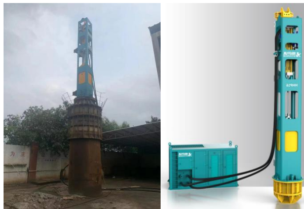
Figure 3: Physical map and actual drawing of hydraulic pile hammer
