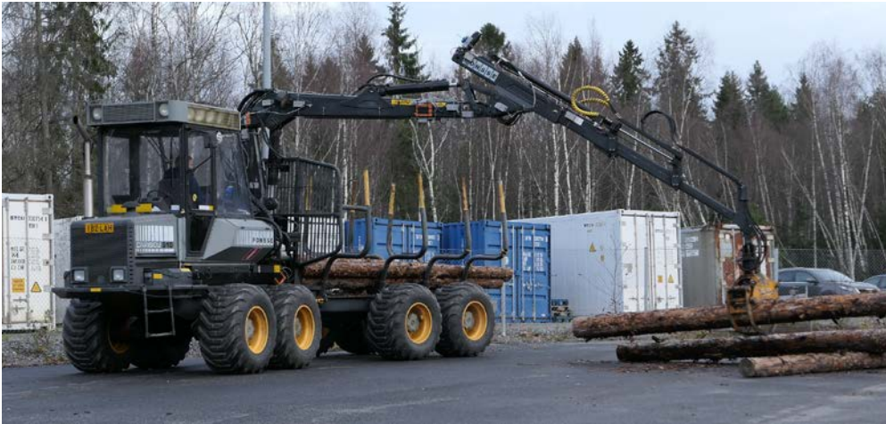
Figure 9: Ponsse Caribou forwarder as a test platform for the pump controller
