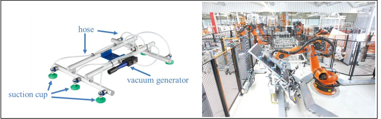
Figure 1: Typical structure of a vacuum handling system and a typical industrial application [7]
