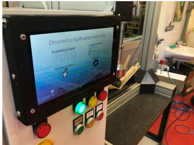
Figure 4: HMI interface of the test device
