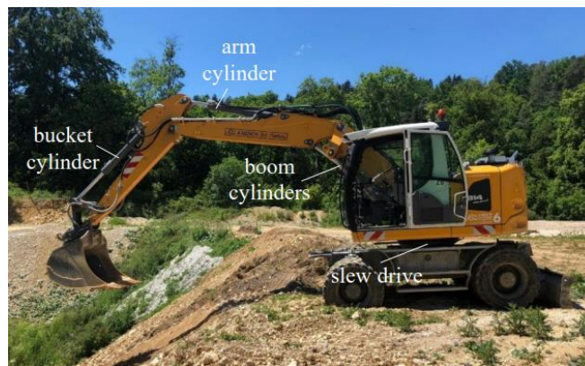
Figure 8: Excavator (Liebherr A 914 Compact Litronic) considered in the modelling
