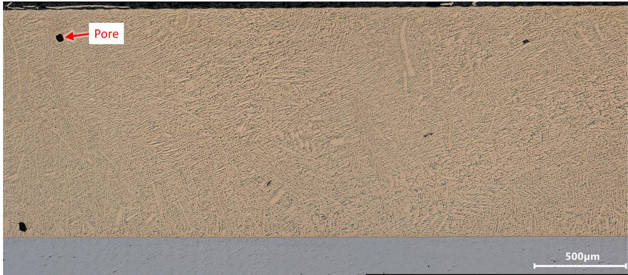
Figure 4: Metallographic cross-section of laser cladded CuSn11Bi3 (Tokat300) on C45 steel
