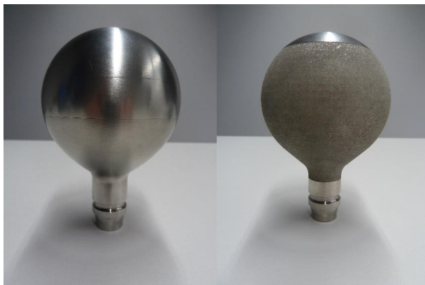
Figure 8: Helmholtz Resonator - conventional and additive manufacturing
