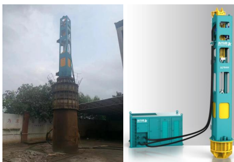
Figure 3: Physical map and actual drawing of hydraulic pile hammer
