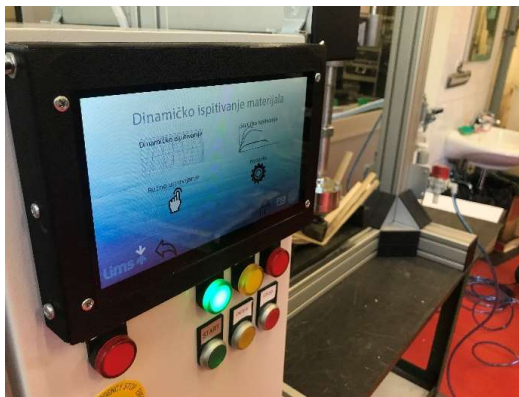
Figure 4: HMI interface of the test device
