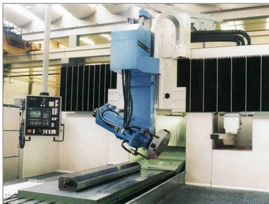
Figure 12: Table, portal and grinding support of machine chosen as application example.
