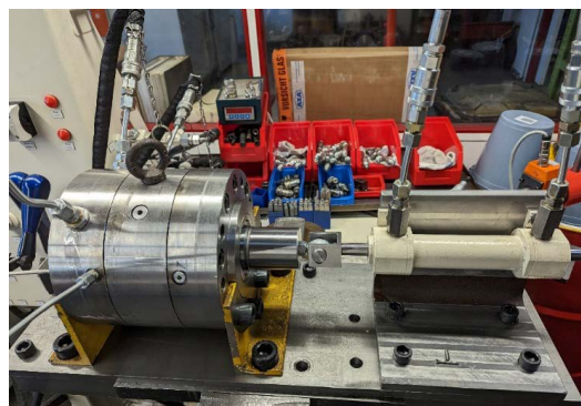
Figure 6: Swivel drive SP 15 D at the test stand for test 1 and 2
