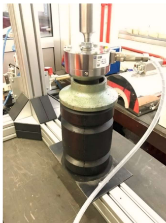
Figure 9: Estimation of process parameters using a rubber bumper
