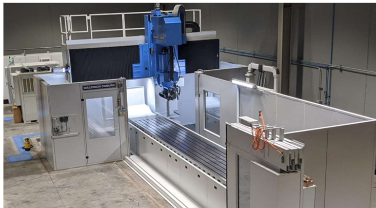
Figure 11: Grinding machine by Waldrich Coburg Company (6 m grinding length)
