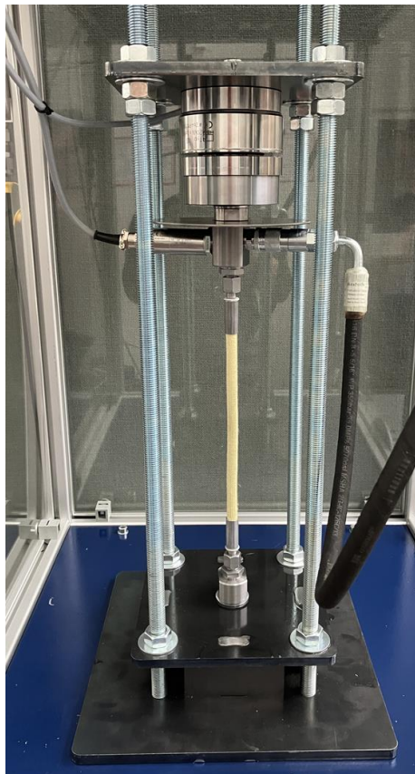
Figure 7: Measuring device to determine the maximum blocked force F_b of the clamped muscle
