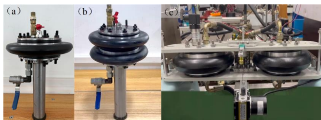
Figure 5: Prototype of the VVPR: (a) Single-layer reservoir (b) Series reservoir (c) Parallel reservoir
