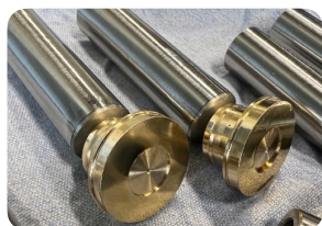
Figure 4: investigated slipper designs and their optimized micro structure
