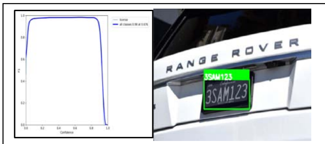
Fig. 6. (a) F1 Score vs Confidence plot for YOLOv5 model; (b) Output of Deployment code after EasyOCR
