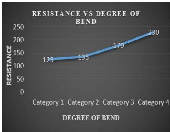
Fig.6.8. Relationship between the variation of resistance and degree of bend.
