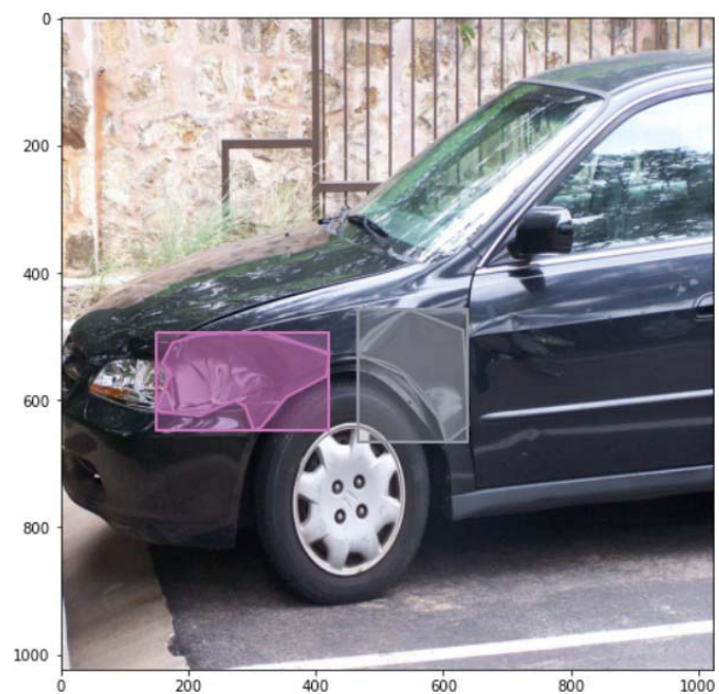
Fig.3. Bounding Box detecting the damage
