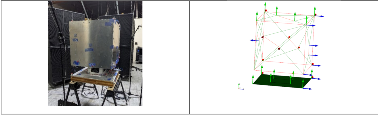
Fig. 3 Test article (left) and test display model with accelerometer measurement degrees of freedom (right).
