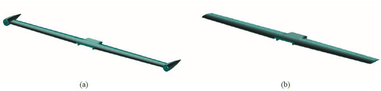
Fig. 5 X-57 Mod III wing finite element model configuration A (Fig. 5a) with the cruise nacelles; and configuration B (Fig. 5b) with only the clean wing.
