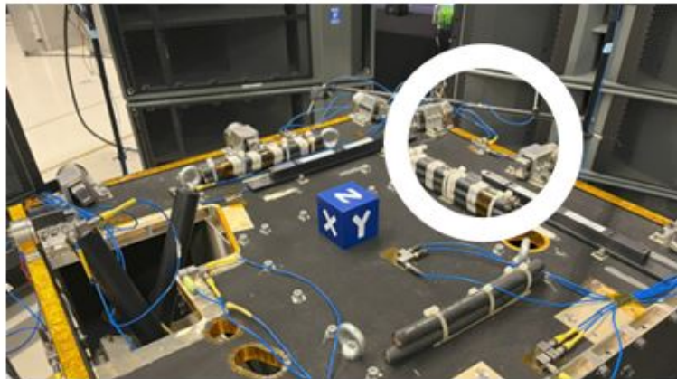
Fig. 13 Location of triaxial reference sensor for OMA. Courtesy of ESA and Redwire Space NV
