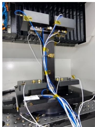
(a) Small Sat Dynamic Simulator with Adjustable Ballast: 3 Mass Configurations for 3 Unique Test Items
