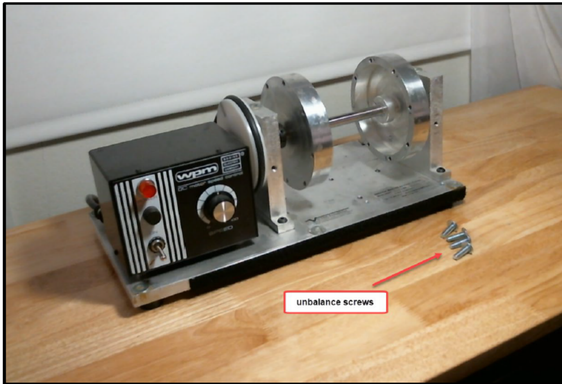
Fig. 1 Rotating Machine Showing Unbalance Screws Added to Its Rotors
