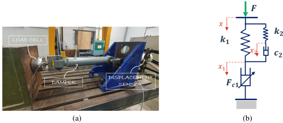
Fig. 1 Experimental bench used for the yaw damper characterization (a). Rheological model of the yaw damper (b).
