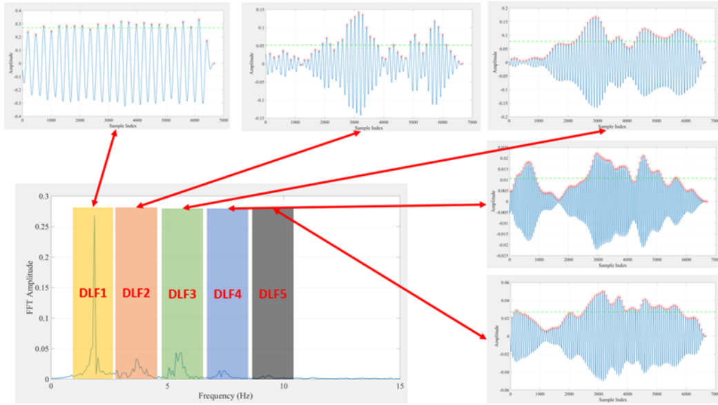
Fig. 4 Modified approach to extract DLF through Time Domain Averaging method.
