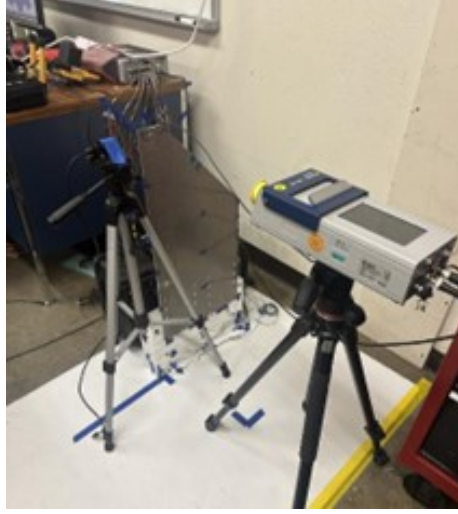
Fig. 7 Comparison setup with LDV and neuromorphic camera.
