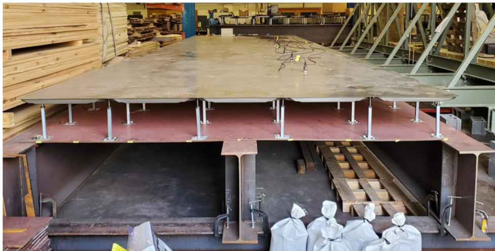
Fig. 1 The light specimen (SM68_RAF) with W24x68 beams, a 3/8 in. thick plate, and raised access floor (RAF).
