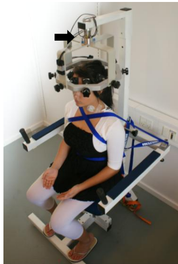
Fig 5: Device used to measure multidirectional isometric neck force. Participants are seated with their head rigidly fixed by 8 contacts in the headpiece. The subject's back and torso are firmly strapped to the seat back. Surface EMG was acquired from SCM and SPL muscles bilateral (SPL electrodes not visible on picture). Arrow point to force transducers based on strain gauges measuring force in coronal and sagittal planes.
