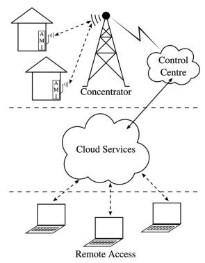
Figure 2 Smart Grid topology including radio communication, cloud services and remote access
