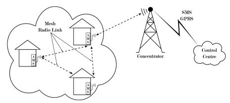
Figure 1 Smart Grid for automatic meter readers
