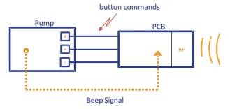
Figure 7.11 Connection diagram between the pump and the designed PCB.
