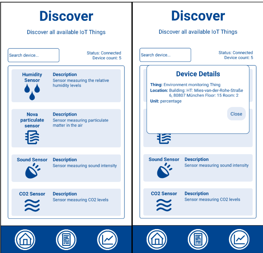
Figure 8.4 TSMATCH client, interface that obtains the available descriptions of existing sensors in an infrastructure in real time.
