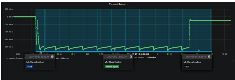
Figure 16.11 Symphony Visualization App displays the behavior of the remote pressure sensor.
