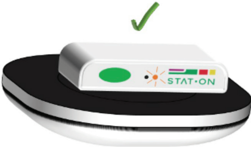
Figure 5.2 Device correctly placed on the charging platform (LED always orange while charging and always off when the charge is completed).
