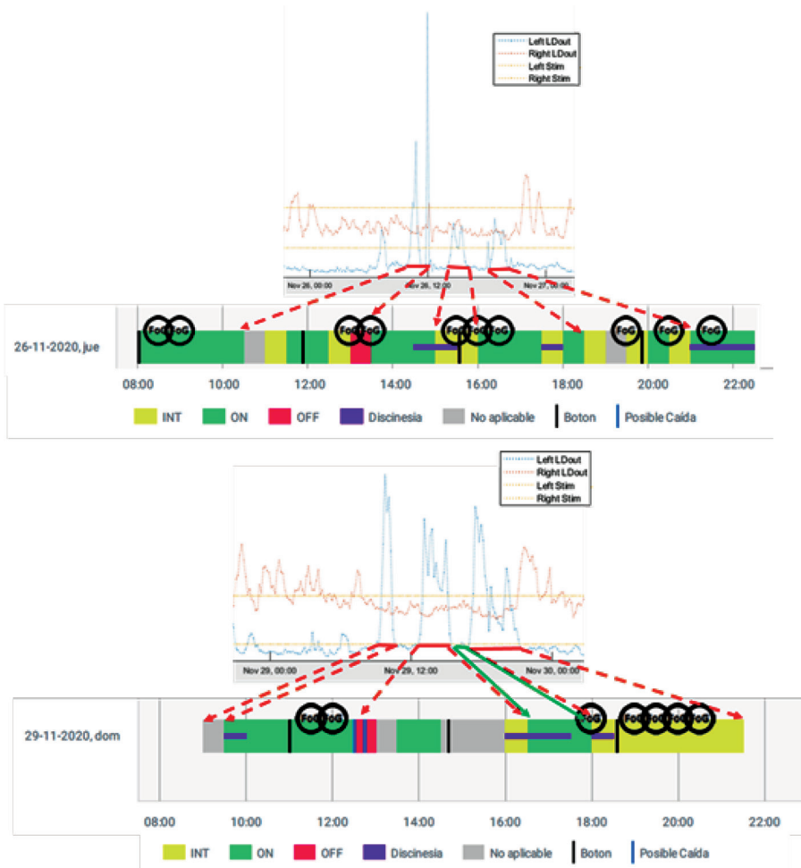
Figure 6.26 Correlation between daily recordings of beta bands and motor status according to Percept™ and STAT-ON™, respectively. Beta bands (blue spikes in the top graph) coincide with OFF (red), “intermediate” (yellow) or “not applicable” (gray = no motion detected) motor status periods detected by STAT-ON™. The ON periods (green) coincide with beta-band free intervals. Most freezing of gait (FoG) episodes detected by STAT-ON™ coincide with non-ON periods.
