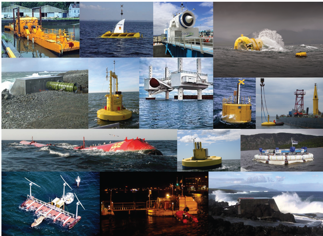
Fig. 1.5. Pre-commercial WECs listed in (Gadonneix et al., 2010), from left to right and from top to bottom: McCable Wave Pump, WavePlane, OceanLinx, Oyster, WaveGen Limpet, OPT Ocean Power Technology, Wavestar, IPS OWEC, SEABASED, Pelamis, SEEWEC, AWS Ocean Energy, Poseidon, OE Ocean Energy, Pico OWC. Only WECs developed in physical models are shown.
