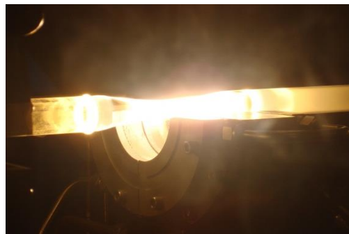
Figure 12 – Collapsing the preform tube
