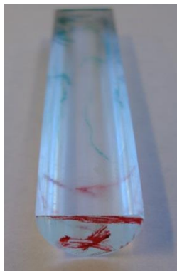
Figure 16 – PA preform milled down to a D-shape
