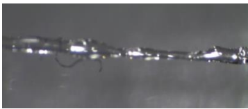
Figure 35 – Uneven recoated LPG
