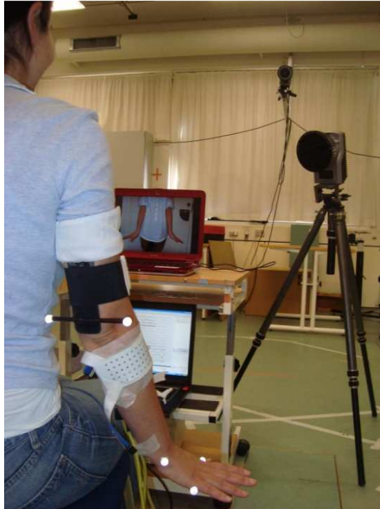
Fig. 4 Experimental setup of Study I. Surface EMG signals were detected from forearm muscles of the right limb and hand kinematics of both limbs was concurrently recorded during the mirrored bilateral movements. The movements to be reproduced were displayed on a computer screen located in front of the subject.
